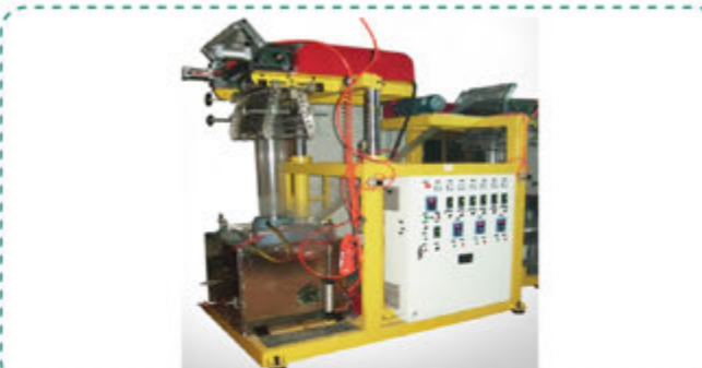
Aluminum PVC Heat Shrinkable Film Upward Blowing Machine Application: aluminum film
