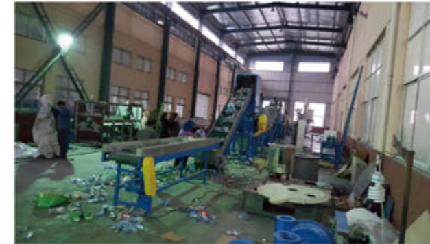
PET bottle crushing, washing and drying line
