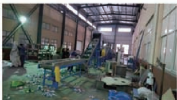
PET bottle crushing, washing and drying line
