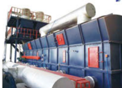
EPS fire retardant coating and drying system
