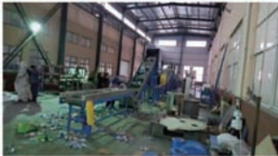
PET bottle crushing, washing and drying line
