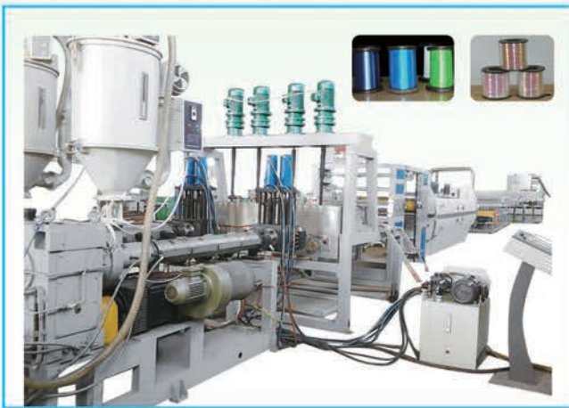
PET/PP高速扁丝曲丝生产线 PET / PP High Speed Flat and Curved Yarn Production Line
