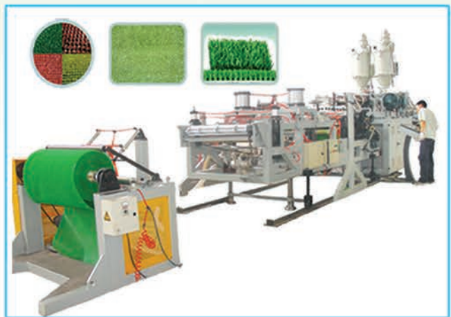
塑料草垫/防飞溅汽车挡泥板生产线 Plastic Grass Mat Production Line
