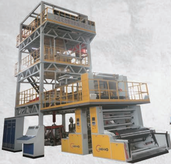
三层共挤HDPE复合膜吹膜机组 3LAYER CO-EXTRUSION BLOW FILM MACHINE FOR HDPE LAMINATION FILM
